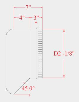
\*38 DIAMETER AND UP 4" AND DOUBLE RIB
